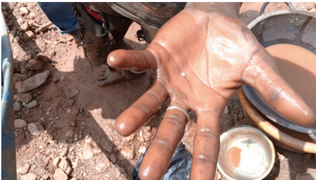
Figure 31: Wet milling and mercury use at gold mining site near Dafa, Abuja state (Photo: Gbenosa 2021)
